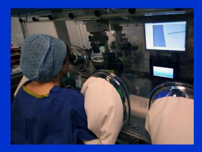
Fully enclosed system protects against temperature and pH fluctuations, and VOCs
