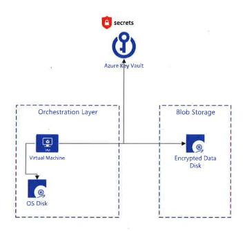
One of the limitations of this approach is it's not scalable for the reason that a disk cannot be shared between two or more instances of virtual machines. For that reason, Orchestration Layer machine can only be scaled up.
