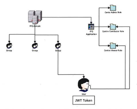
IFQ Application (see diagram below) is registered in IFQ domain. In terms of AAD application is a separate entity which can hold application specific roles and control user access separate to the primary domain. Application also allow to control directory access in a finer grained way comparing to using the global directory.
